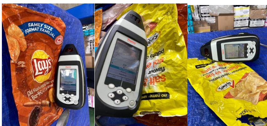
Figure 2 – Example of chip bags identification with a resin identification device
