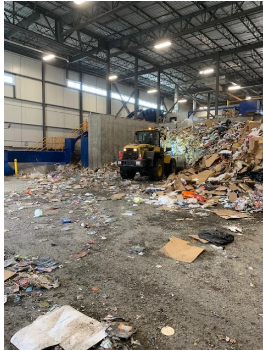
Figure 11 Tipping floor (Société Via, Qc.)
