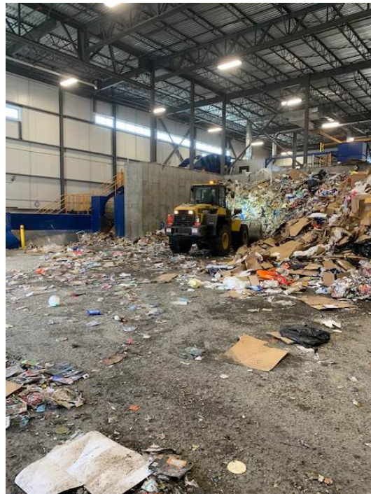
Figure 11 Tipping floor (Société Via, Qc.)
