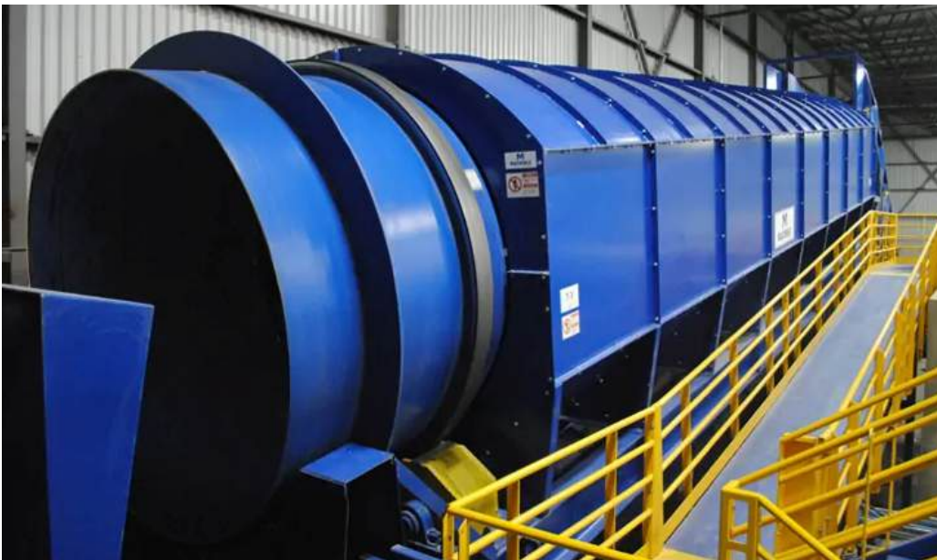
Figure 24 Machinex Trommel (C)
