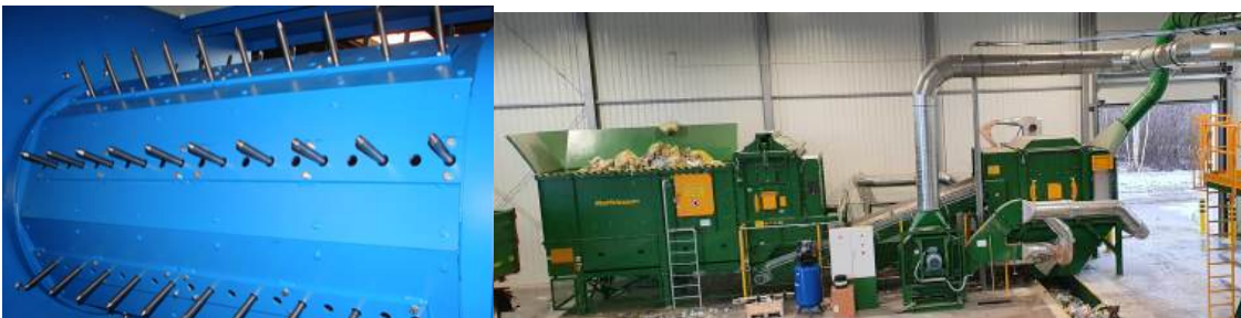
Figure 25 Matthiessen Oversize separator combined with a bag ripper and air separation (D)
