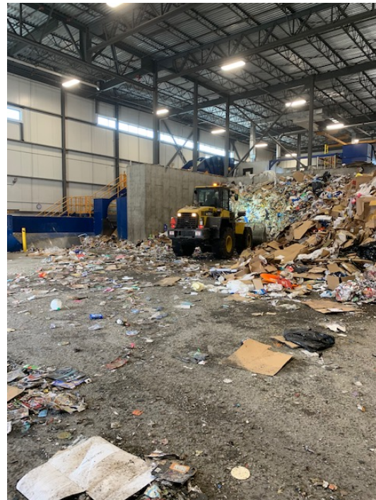
Figure 11 Tipping floor (Société Via, Qc.)
