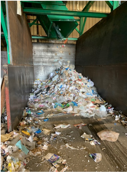
Figure 14 FPP and other material rejected from 2D fibre line (Mazza Recycling, NJ)
